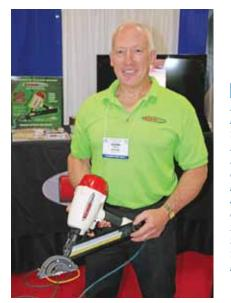
Decking pros got new options at the show too. HID Fast's new Edge Fast hidden fastener decking nailer drives nails at a 35-degree angle into wood and composite boards for a clean, invisible fastener look with the speed of an air nailer.
