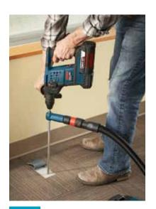
When used with a dust collection system, Bosch hollow core Speed Clean bits virtually eliminate dust at the source for faster, safer drilling and far less job site clean-up.
